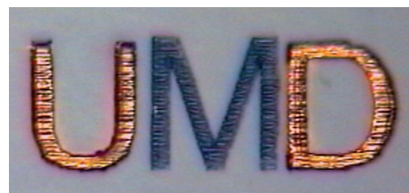
Figure 9. Selective metallization of microstructures created with MAP. The “U” and the “D” were created from an acrylic polymer and the “M” from a methacrylic polymer. Copper was deposited selectively on the acrylic structures.
